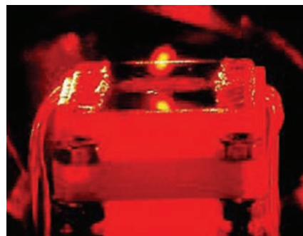
ATOM CHIP in the lab of Jörg Schmiedmayer at the University of Heidelberg traps a cloud of cold lithium atoms above its surface. The mirror image of the atom cloud is visible in the chip's shiny gold-coated gallium arsenide surface.
