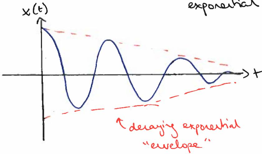
$\omega = \sqrt{\underbrace{\frac{k}{m}}_{\omega_0^2} - \underbrace{\left(\frac{b}{2m}\right)^2}_{\text{damping term}}}$
