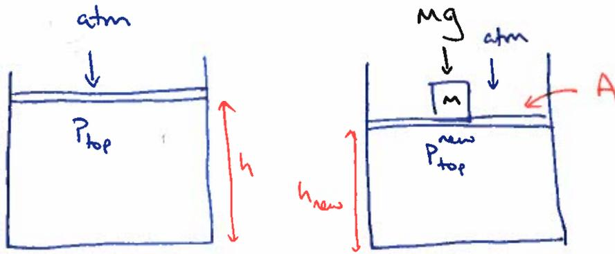
$$\Delta P_{\text{top}} = \frac{mg}{A} \quad \text{due to mass } m \text{ exerting force } mg \text{ over area } A$$
