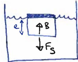
$$B = \rho_{\text{H}_2\text{O}} V_{\text{H}_2\text{O}} g = \rho_{\text{H}_2\text{O}} e^3 g$$
