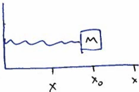
If we treat the spring as part of the system, then compressing or extending the spring stores potential energy in the system.
