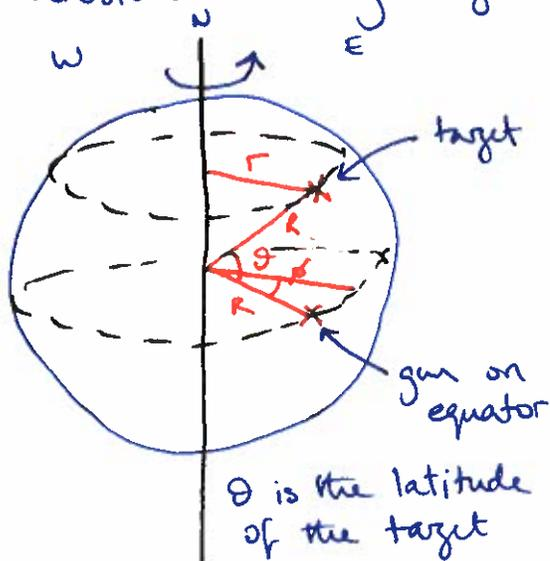
The gun is moving (in an inertial frame)
